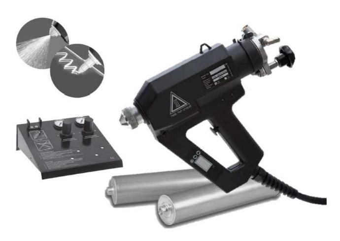
The spray system AS-5080-P-LCD allows the handling of high- and low viscous PUR-hot melt adhesives in 310ml AL cartridges without the usage of any dissolver. The application can be dots or line type.
